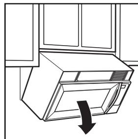
6. Lift off the support tabs **F** at the bottom of the mounting plate. Set the microwave oven aside on a protected surface.
